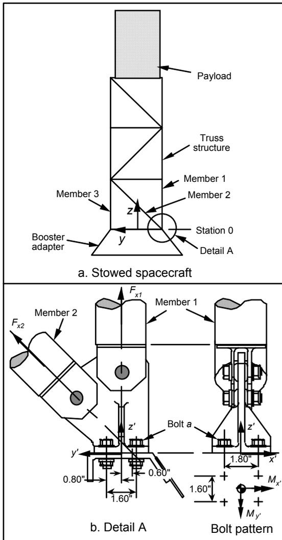
**Fig. 4. Hypothetical Spacecraft and Area of Concern.** The objective is to devise a static load case that will develop the design limit tensile forces in member 1 and in bolt a.
