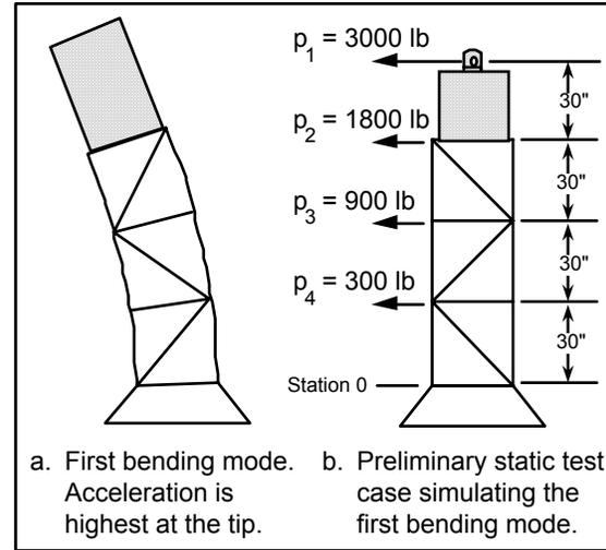
Fig. 5. **Simulating the Example Spacecraft's First Bending Mode with a Preliminary Load Case.** Load magnitudes were chosen to be approximately proportional to the mode shape's displacements while also causing a bending moment at station 0 equal to the design ultimate load of 585,000 in-lb. For this example, mass is assumed to be uniformly distributed along the spacecraft's length.
