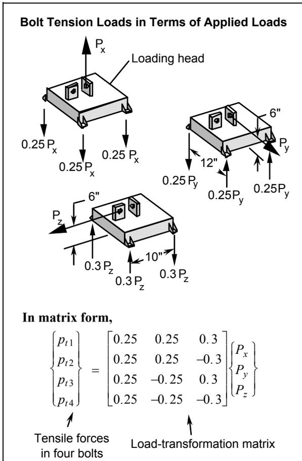
**Fig. 3. Simple Example of a Load-Transformation Matrix.** This matrix relates bolt loads to applied loads. We can also relate bolt loads (or stresses) to modal responses computed in loads analysis.
