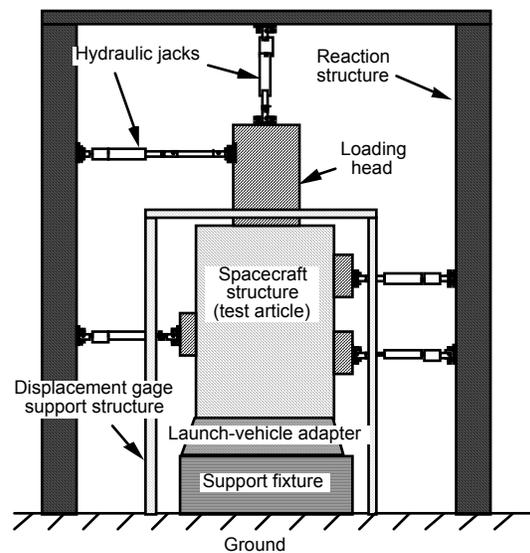
Fig. 1. Typical Configuration for a Static Test with Hydraulic Jacks.
