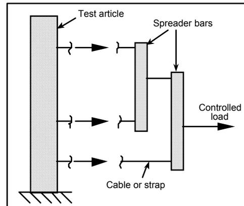
**Fig. 6. Example Whiffletree for Distributing Loads.** Each spreader bar is statically determinate.
