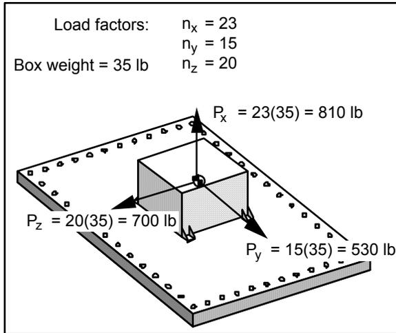
**Fig. 2. Example Structure that will be Statically Tested.** The objective is to verify the panel’s strength for the design limit loads shown.
