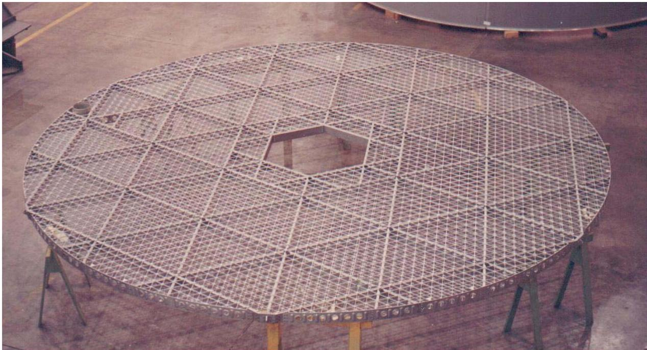
**Fig. 20-1. Open Isogrid Lattice Used for Skylab.** This is a photo of a floor assembly that was 21 feet in diameter. The isogrid design is analogous to a pegboard, with each node providing an attachment point.
