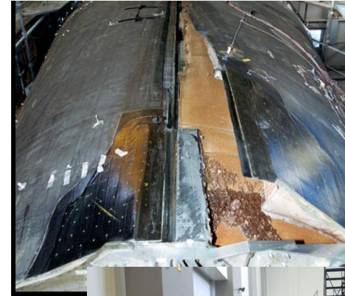
X-33 liquid hydrogen tank test failure, Nov. 1999
