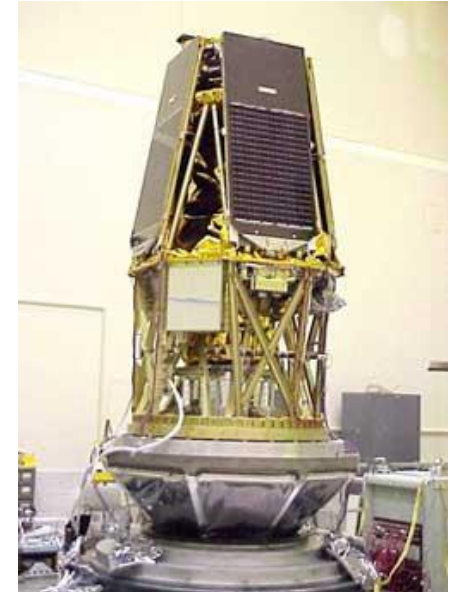
HESSI after repair. The test in March 2000 that caused the failure was lateral, on a slip table.
