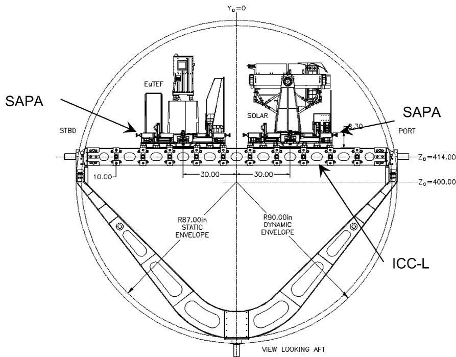
Fig. 1 ICC-L, EuTEF, and SOLAR looking aft in the Orbiter cargo bay, with the 87-in. static and 90-in. dynamic cargo envelopes depicted:  $Y_0 = 0.0$  and  $Z_0 = 400.0$  define the cargo envelope centerline.
