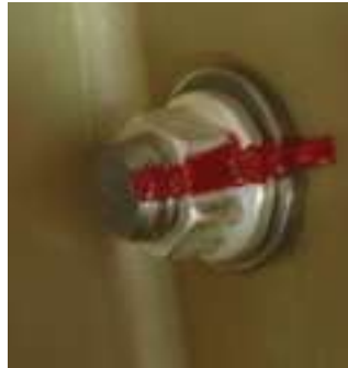
Fig. 3-3. Torque Striping. The stripe is painted after the nut is torqued. After vibration testing, a break in the stripe between the nut and the end of the bolt indicates relative rotation between these parts, hence preload loss. For a screw going into a blind hole, the stripe must continue onto the clamped structural part, as shown above for the nut. (Image from americanprecisionassembly.com)
