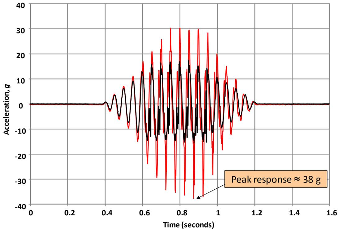
**Fig. 4-10. Response Measured at the Top of the Spacecraft Structure, Superimposed With the Input Acceleration from Fig. 4-9.** The 60-Hz input excited the 62-Hz response mode, causing 38 g peak response as compared to a target of 15 g uniform acceleration.
