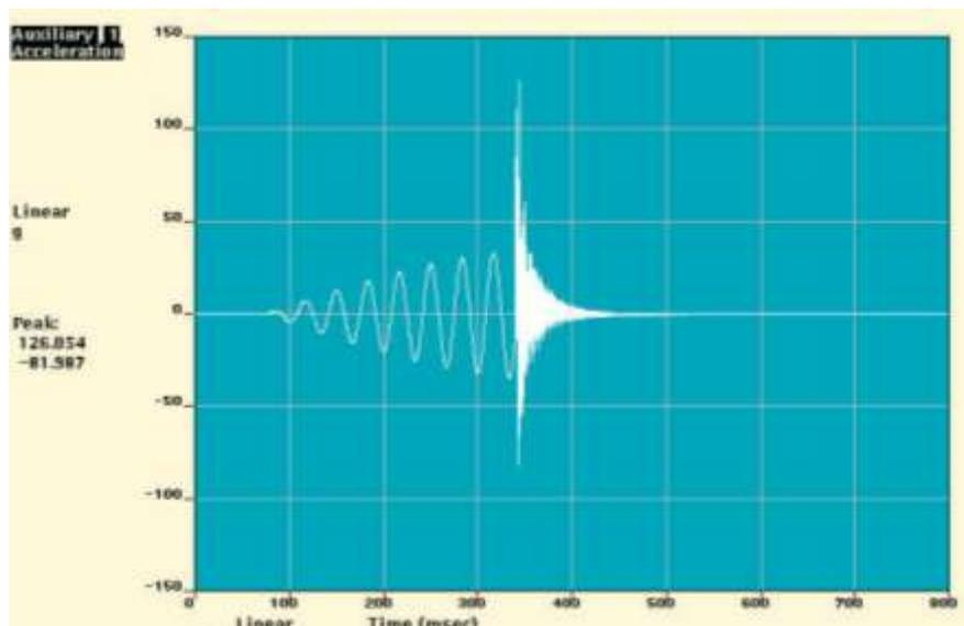
**Fig. 4-12. Response Measured at the Top of a Test Article During a Failed Attempt at a Sine-Burst Test.** The high sudden response was attributed to failure of the shaker’s amplifier. Fortunately this test was conducted on a low-cost engineering model of a spacecraft structure!
