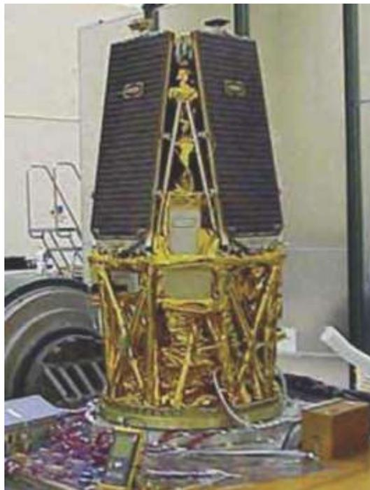
**Fig. 4-13. High Energy Solar Spectroscopic Imager (HESSI) Spacecraft on Shaker.** This photo was taken at JPL in March 2000 shortly before the sine-burst test anomaly that did over one million dollars of damage to the spacecraft. In the initial low-level (-12 dB) run, the slip table did not move freely and then suddenly let loose, with approximately 21 g acceleration, whereas the target acceleration was 1.88 g. (Image courtesy NASA Jet Propulsion Laboratory, from Ref. 3)
