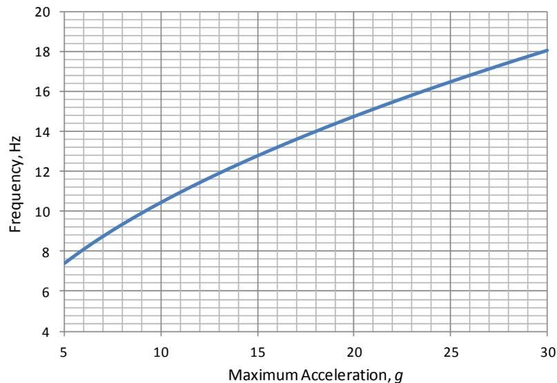
**Fig. 4-8. Recommended Minimum Sine-Burst Frequency vs. Desired Maximum Input Acceleration for a Shaker with a Two-Inch Stroke, Peak to Peak.** This plot includes the 0.9 reduction factor, per Eq. 4.6.
