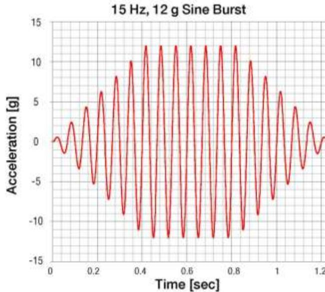
Fig. 4-1. Example Input Acceleration for a Sine-Burst Test.
