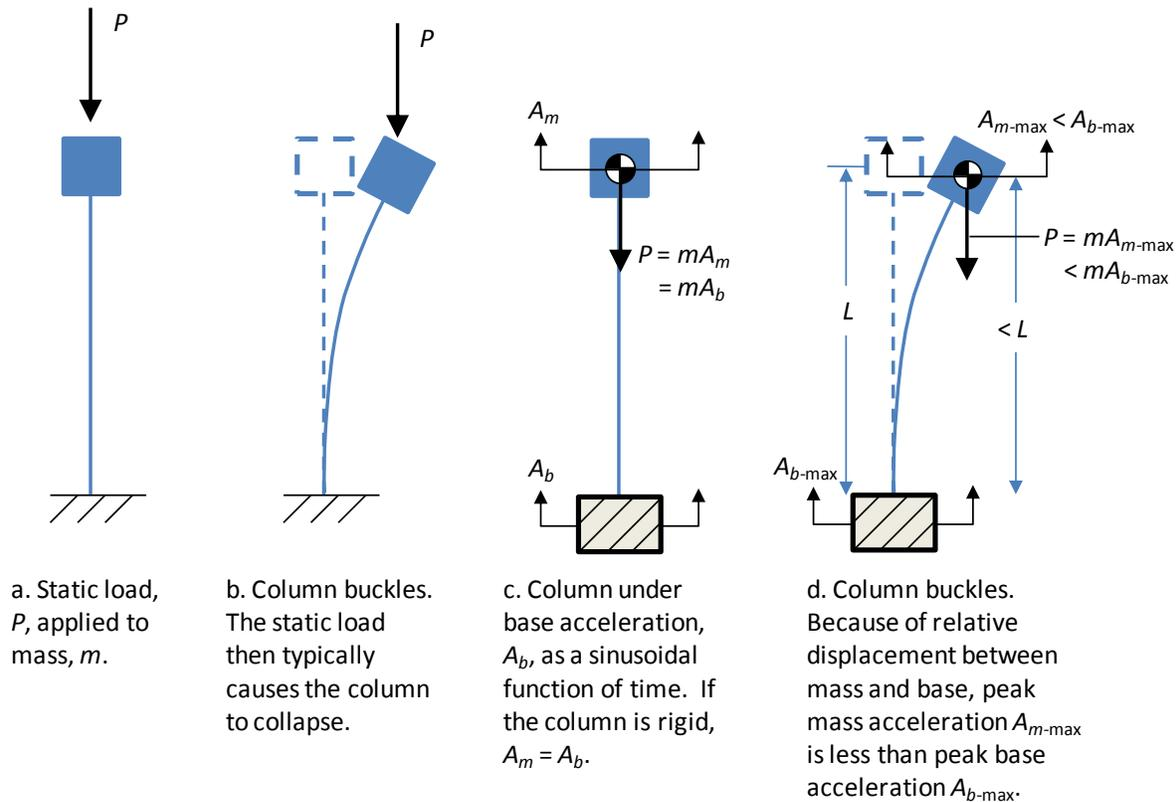
**Fig. 4-2. Buckling of a Column in a Sine-burst Test.** A column that would buckle and collapse under a static load may not collapse under a sinusoidal base acceleration that is intended to cause the same peak load.
