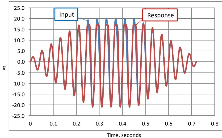
**Fig. 4-3. What the Response Might Look Like if the Structure Starts to Buckle.** If any mass within the test article does not see acceleration that is at least as high as the input acceleration, part of the structure may be buckling or yielding. Here, the structure may be buckling at about 17 *g*.
