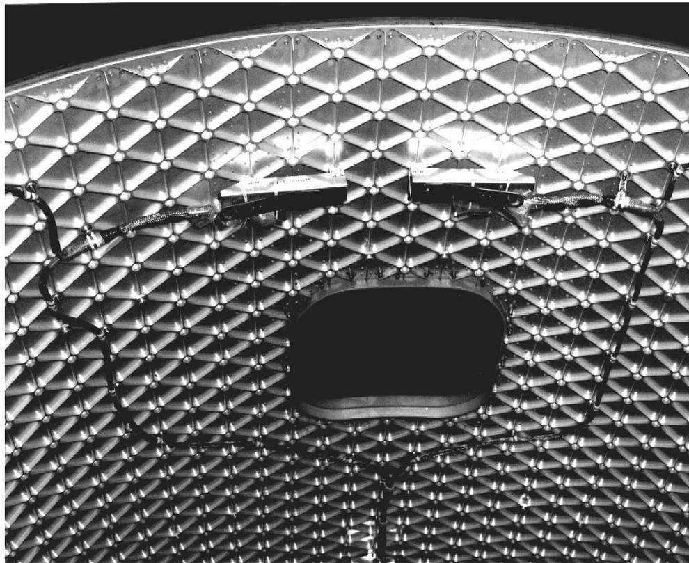
**An integrally machined isogrid structure provides an attachment point at each node—a pegboard—allowing the structure to adapt to late-added components.**
