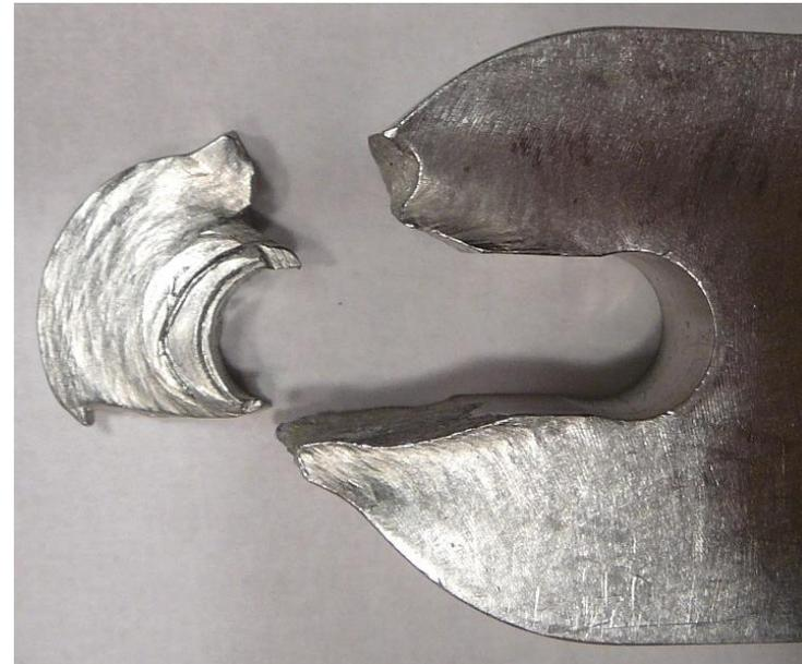
The material can undergo very large plastic deformation, elongating the hole.
