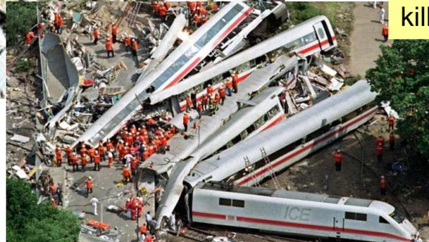
1998 derailment of high-speed train near the village of Eschede, Germany, as a result of fatigue failure of a wheel, killing over 100 people
